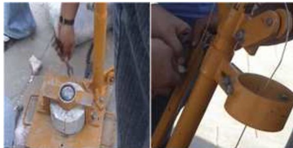
Figure 12: Drop-Weight Hammer Test Setup
